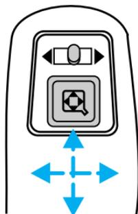
3. Return to the center position to lock mirrors in place.
