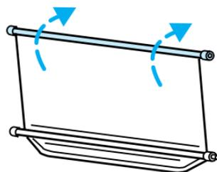
4. Push in the right end cap (marked RH) about  $\frac{1}{4}$  of the total length to disengage the clutch and hold the end cap in while turning the roller tube toward you 14 times.
