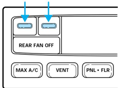
For continuous maximum cooling, push the blue button until 16°C (60°F) is shown in the display window. The EATC will continue maximum cooling (disregarding the displayed temperature) until a warmer temperature is selected by pressing the red button.
