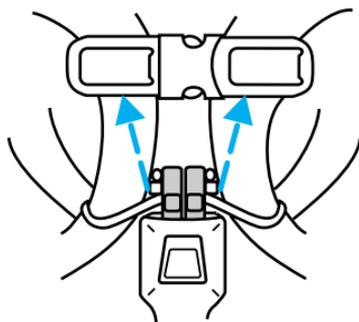
If necessary, the shoulder belt may be put in automatic locking mode (ALR) to limit the child's movement in the seat. The ALR mode should be used if the child is sleeping or attempting to get out of the seat.
