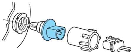
2. Slip the bulb retaining ring over the plastic base until it contacts the rear of the socket by rotating it clockwise until you feel a “stop”.
