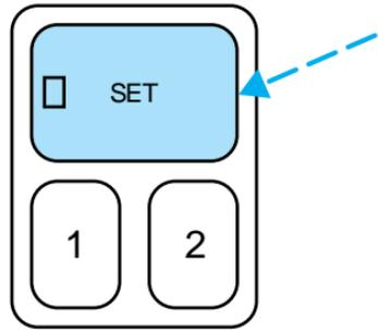
A position can only be set or recalled when the transmission gearshift is in Park or Neutral. A memory seat position may be programmed at any time.
