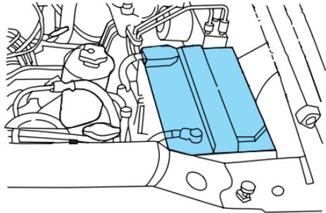
If the electrolyte level in the battery is low, you can add plain tap water to the battery, as long as you do not use hard water (water with a high alkali content). If possible, however, try to only fill the battery cells with distilled water. If the battery needs water often, have the charging system checked.
