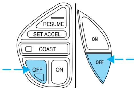
Once speed control is switched off, the previously programmed set speed will be erased.
