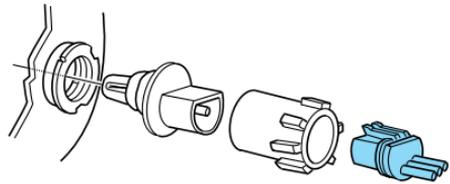
4. Remove the bulb retaining ring by rotating it counterclockwise (when viewed from the rear) about an eighth of a turn to free it from the bulb socket, and by sliding the ring off the plastic base. Keep the ring because it will be used again to retain the new bulb.
