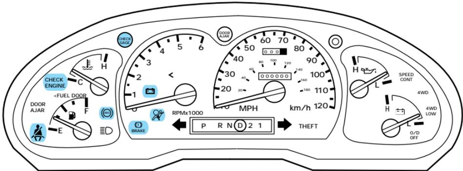
Make sure the corresponding lights illuminate briefly. If a light fails to illuminate, have the vehicle serviced.
