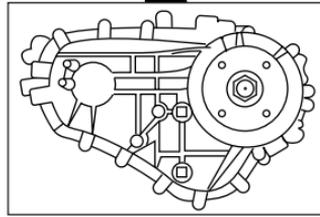
3. Add only enough fluid through the filler opening so that the fluid level is at the bottom of the opening.
