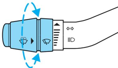
Push the control on the end of the stalk to activate washer. Push and hold for a longer wash cycle.
