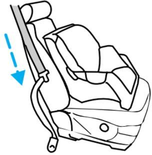
3. While holding the shoulder and lap belt portions together, route the tongue through the child seat according to the child seat manufacturer's instructions. Be sure the belt webbing is not twisted.
