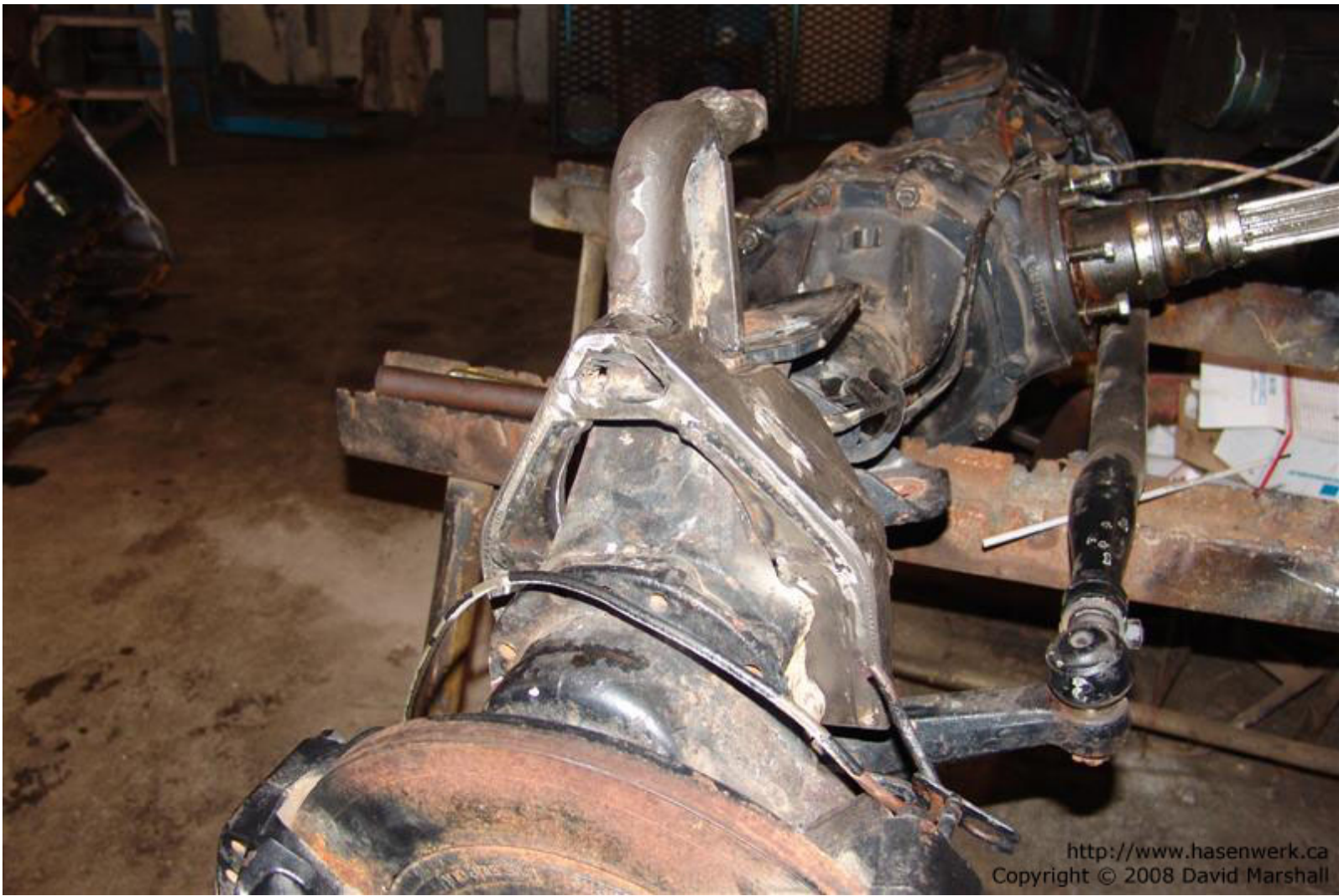
Volksmogen steering arm built from a Ford F350 steering arm and heavy plate steel
