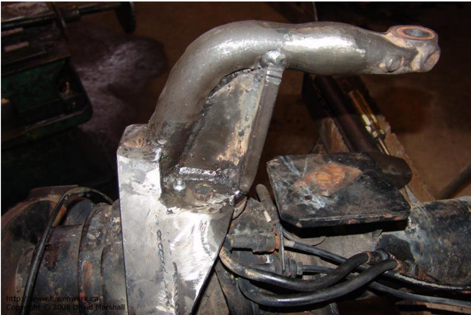
Volkswagen steering arm built from a Ford F350 steering arm and heavy plate steel
