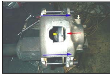
Operation of a Floating Calliper
