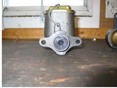
Input side of the master cylinder piston.
