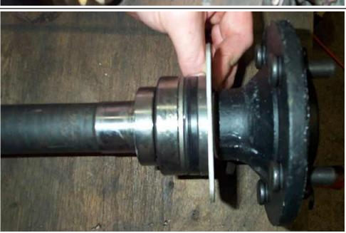
Here's the new seal, bearing, and locking ring installed on the shafts. Note the custom steel machined spacer between the bearing backing plate and the seal....part of my ZJ rear disc conversion, detailed elsewhere on my site.
