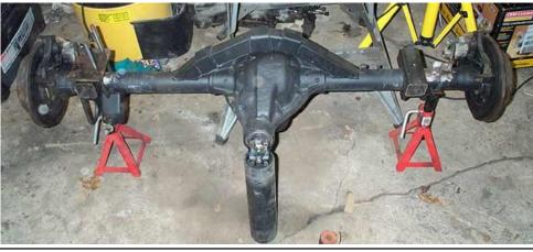
Complete with ZJ rear disc brakes, custom truss and spring perches, and ready to install.
