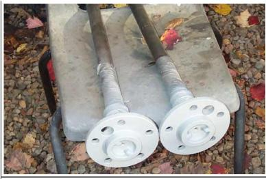
Shafts removed, cleaned, and primed.
