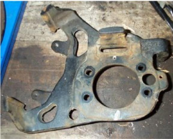
The bracket, ready to go to the welders / machine shop. You need someone experienced with cast steel to do the welding.
