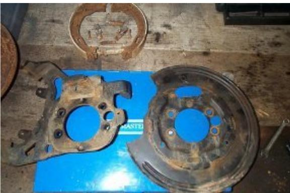
The splash shield and caliper mounting bracket separated.
