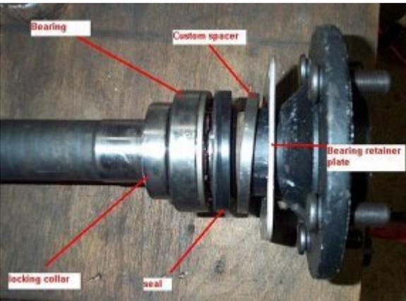
Here's the arrangement of parts on the axle, including the custom spacer in place.
