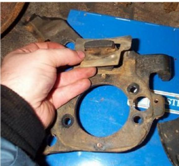
Once you remove the splash shield, you have to remove the little rubber e-brake lever boot.
