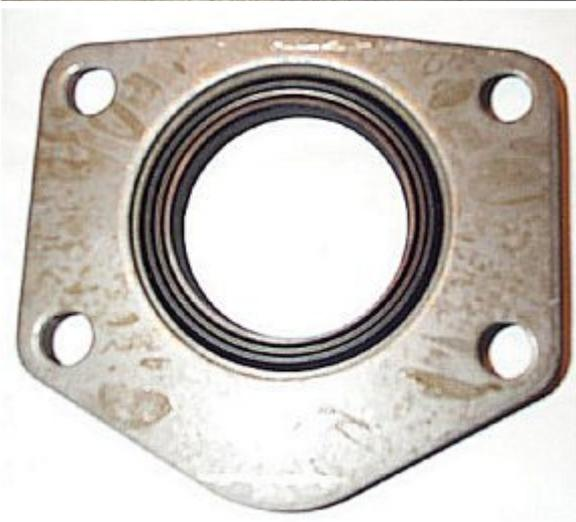
The stock configuration of the bearing retainer plate against the axle seal.
