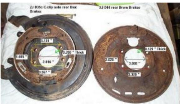
This shows the difference. The center will need to be reamed out, the bolt pattern welded and re-drilled to match, and a custom spacer (next pic) machined to fit on the shaft outboard of the axle seal, to ensure the bearing sits in the race properly. Note that the D35 NON c-clip axle bearing retainer bolt pattern is identical to the D44, and so if you copy what I did you can fit the ZJ discs on your d35 non c-clip the same way.
