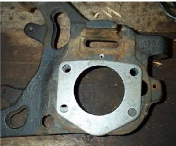
The XJ D44 bearing retainer plate overlaid on the caliper mounting bracket - showing the difference in flange bolt pattern, and the need to weld up and re-drill the caliper bracket.
