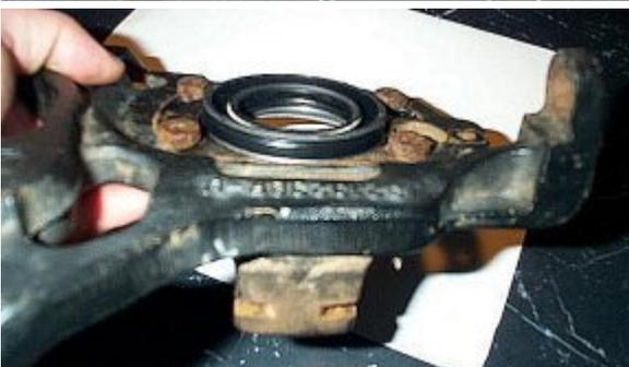
Side view of the seal on the spacer.
