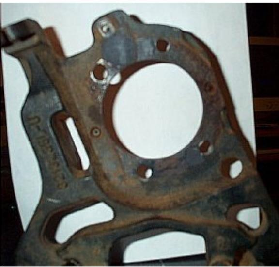
The machine shop swore I'd have no problems as it was, but I just couldn't leave it, so I plugged the hole with a steel putty, 18, 000 psi compression strength.
