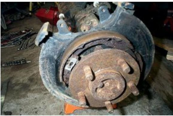
Caliper and rotor removed, e-brake shoes visible.
