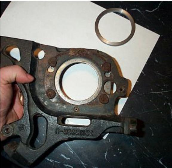
Bearing retainer in place, and custom spacer in background.
