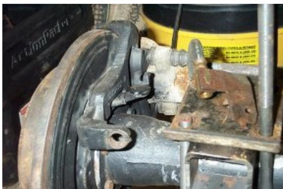
One last mod - I had to weld the XJ drum brake parking brake lever cable fitting end onto the new lever (the ZJ has different cable ends). You could just get ZJ cables, but I'm using the long YJ cables.
