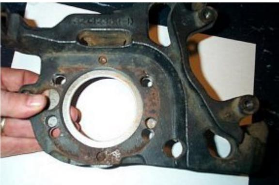
The machine shop wouldn't weld the cast bracket. Luckily it could be re-drilled without welding.
