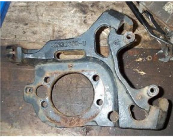
Back of the separated caliper mount bracket. The larger hole to the left side is the hole for the ABS sensor (not used by me)
