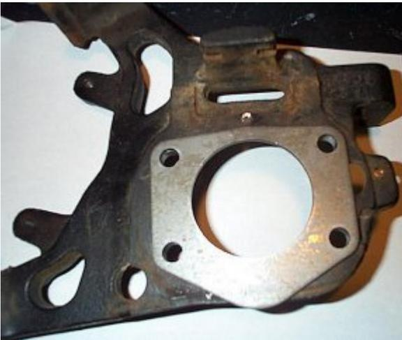
Bearing retainer plate on the re-drilled bracket.
