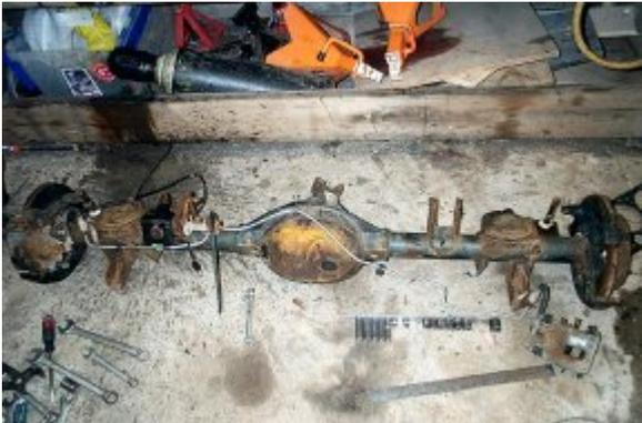
The ZJ D35 axle I bought. It has c-clip axles and 3.55 gears (open).
