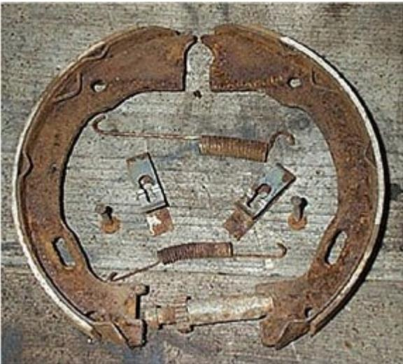
The e-brake shoe assembly removed.
