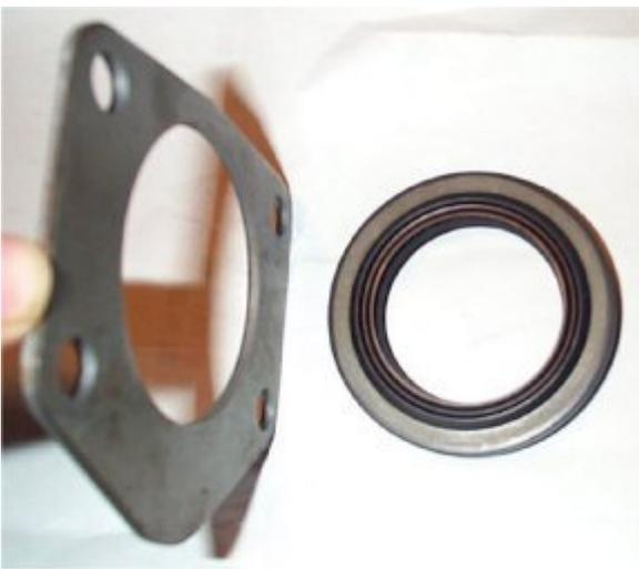
The stock configuration of the bearing retainer plate against the axle seal 2.
