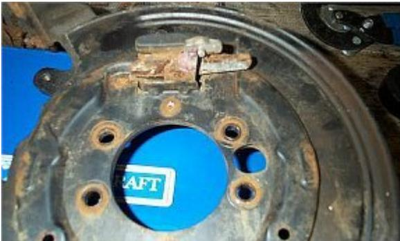
The arrangement of the little e-brake lever.
