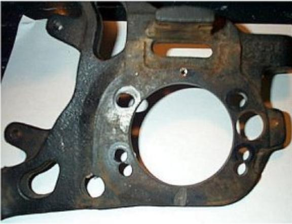
The bracket back from the shop, large hole enlarged to 3", and the D44 bolt pater drilled. They would not weld the cast bracket.
