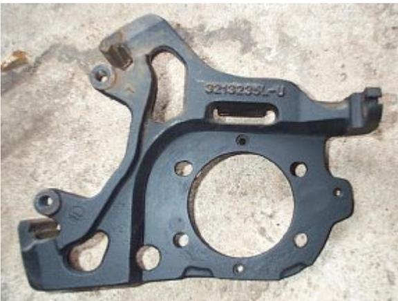
The NEW Dana 44 Disc Brake caliper bracket!
