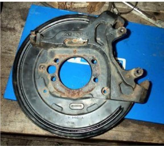
Back of the ZJ disc caliper bracket and splash shield.
