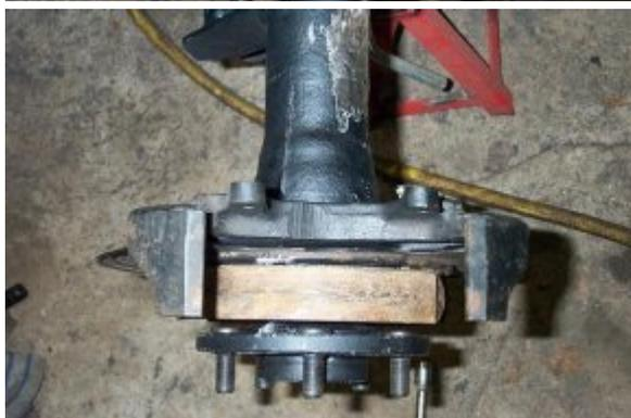
Bracket and brake shoes in place, axle installed. ]
