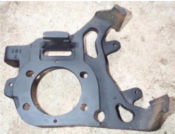
The NEW Dana 44 Disc Brake caliper bracket!
