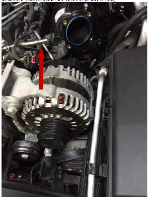
7. REMOVE BELT FROM ALTERNATOR PULLEY (USE 1/2" DRIVE RATCHET ON TENSIONER PULLEY)
