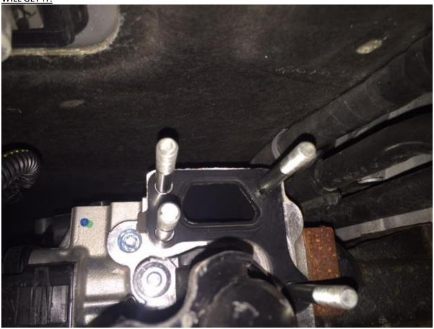
34. REMOVE COOLANT HOSES FROM THERMOSTAT HOUSING
