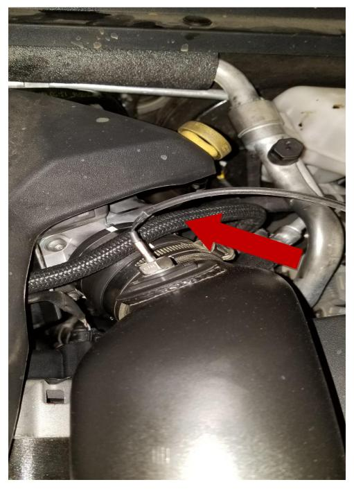
6. DISCONNECT FUEL FEED LINE (3/8" FUEL LINE REMOVAL TOOL)
