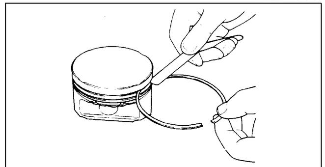
2. Insert the piston ring into the cylinder by hand and use the piston to push it to the bottom of the ring travel.
