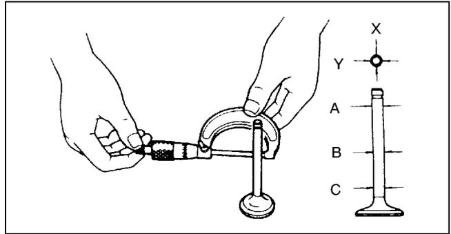
4. Measure the inner diameter of each valve guide in X and Y directions at the three points (A, B, and C) shown. Replace the valve guide if necessary.
