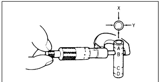
5. Calculate the clearance between connecting rod small end and piston pin. Replace the connecting rod or piston pin if necessary.
