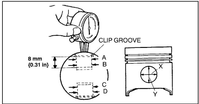
2. Measure each connecting rod small end inner diameter in X and Y directions as shown.
