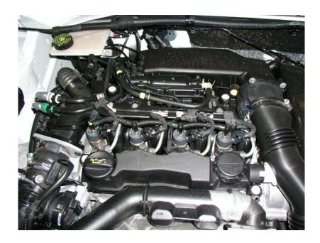
When basic checks have been completed (low pressure fuel supply, interrogate for DTC's, check for fuel contamination etc.), a quick health check of the high pressure fuel system can be done using the graphing function of a scan tool to evaluate live data values for rail pressure and engine speed during cranking, idle and snap acceleration. The fuel rail pressure sensor of a healthy system produces a characteristic waveform which forms the basis for this check.
