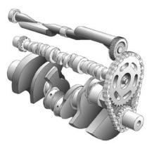
A counter-rotating balance shaft cancels the primary engine vibrations found in 90° V6 engines. The result is smooth performance and low noise.
